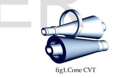
A cone CVT varies the effective gear ratio using one or more conical rollers. The simplest type of cone CVT, the single-cone version, uses a wheel that moves along the slope of the cone, creating the variation between the narrow and wide diameters of the cone. The more sophiticated twin cone mesh system is also a type of cone CVT.
